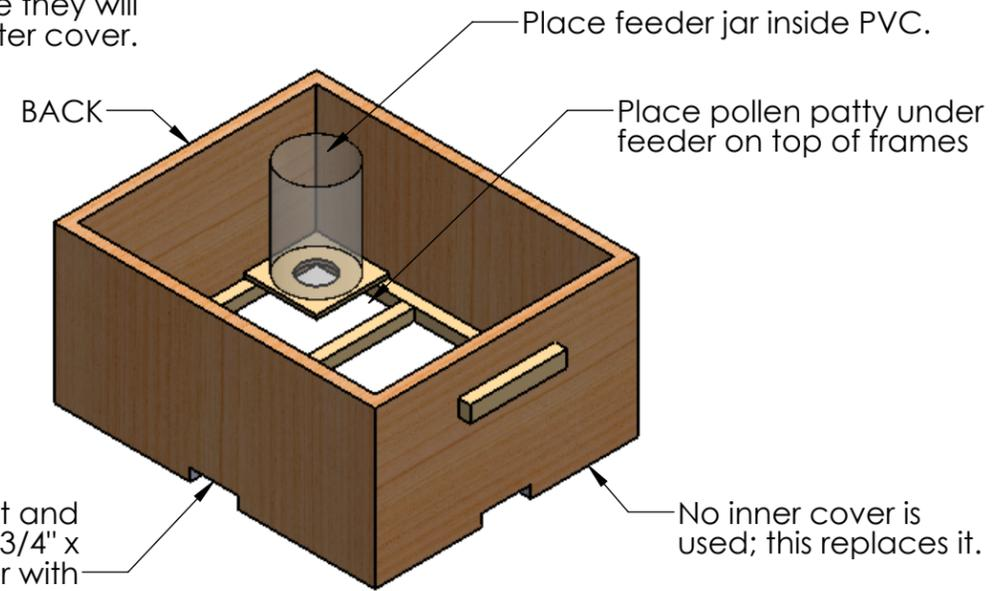
Cut openings in front and sides for air flow, 3/4" x approx 2" and cover with 1/4" to 1/2" hardware cloth to keep mice out.
